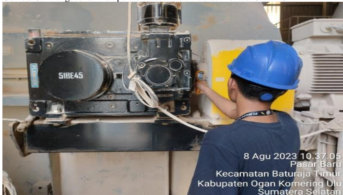
Gambar 3.4 Pengecekan Temperatur mesin Belt Bucket Elevator 51BE45
