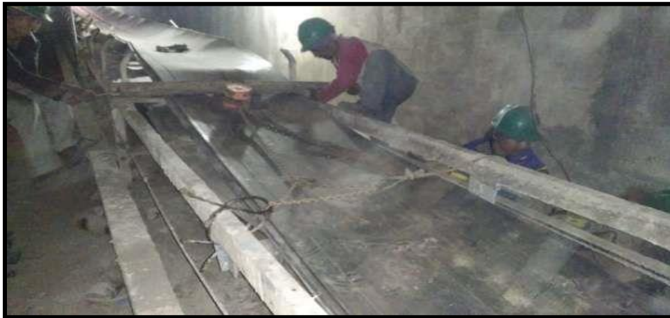
Gambar 4 Pasang Clamp Belt & Ankat Take-Up Pulley
